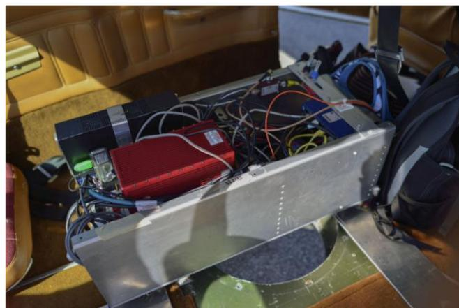
G-LiHT sits inside the airplane's cockpit, over an open camera port that allows it to look down from about 1,000 feet high.
