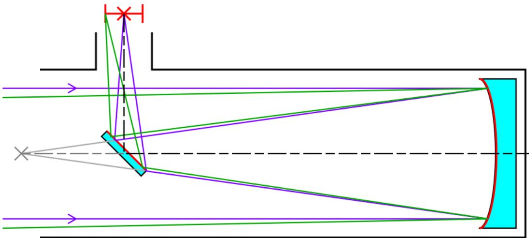
*A diagram of a Newtonian Reflector*
